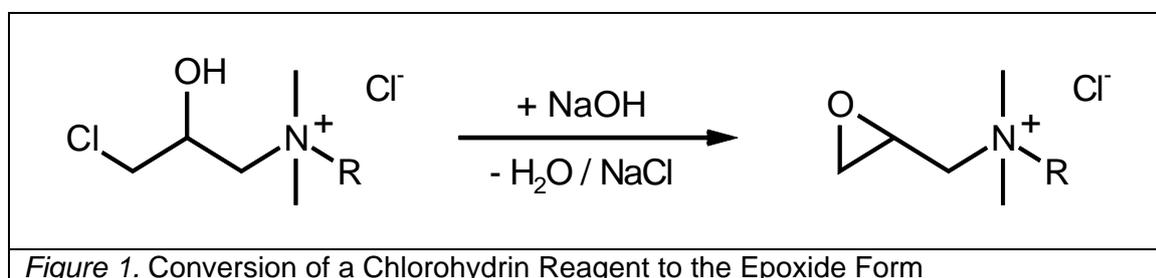
If the reagent used is in the chlorohydrin form, then equimolar quantities of sodium chloride and water are generated as reaction by-products. Some producers of cationizing reagents offer the EPTAC type product, which already exists in the reactive epoxide form. Using such EPTAC cationizing reagents circumvents the formation of salt during the cationization process, but usually at somewhat higher cost.
