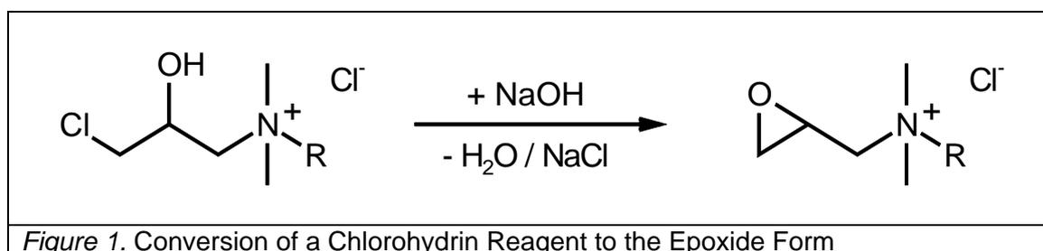
Figure 1. Conversion of a Chlorohydrin Reagent to the Epoxide Form
